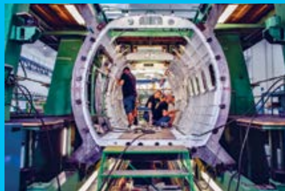
FROM LARGER PIECES, THE ENTIRE AIRCRAFT IS ASSEMBLED
